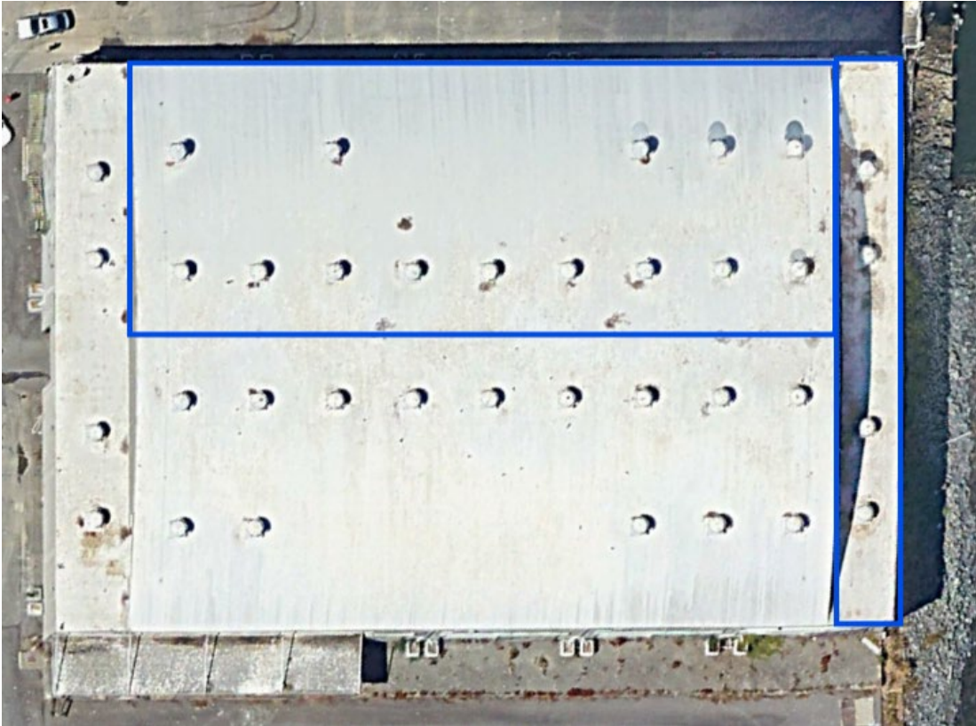
Image 1. Roof vents on Warehouse 1. Area draining to Basin W1C is shown in blue.
