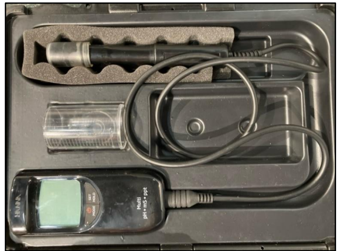
Figure 2- Example instrument, Hannah instruments Portable pH/EC/TDS Temperature device
