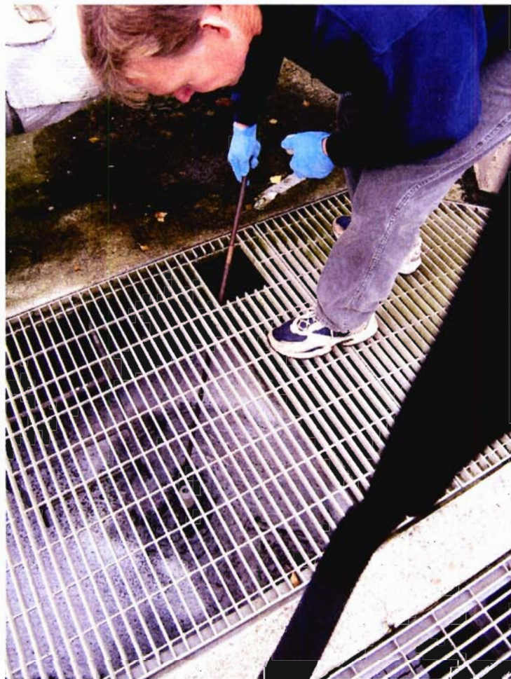
PHOTO #:017 DATE: 10/18/05, 10:18 AM FILE: MCKONE/PA180004.JPG TAKEN BY: SHAWN MCKONE DESCRIPTION: GRAB SAMPLING OF FINAL EFFLUENT AT DISCHARGE END OF CHLORINE CONTACT CHAMBER, RBC PLANT.
