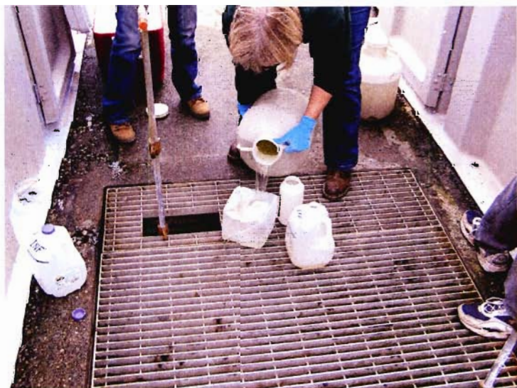
PHOTO #:020 DATE: 10/18/05, 10:02 AM FILE: SMITH/PA180006.JPG TAKEN BY: JARON SMITH DESCRIPTION: SAMPLE SPLITTING, LAGOON COMPOSITE SAMPLES.
