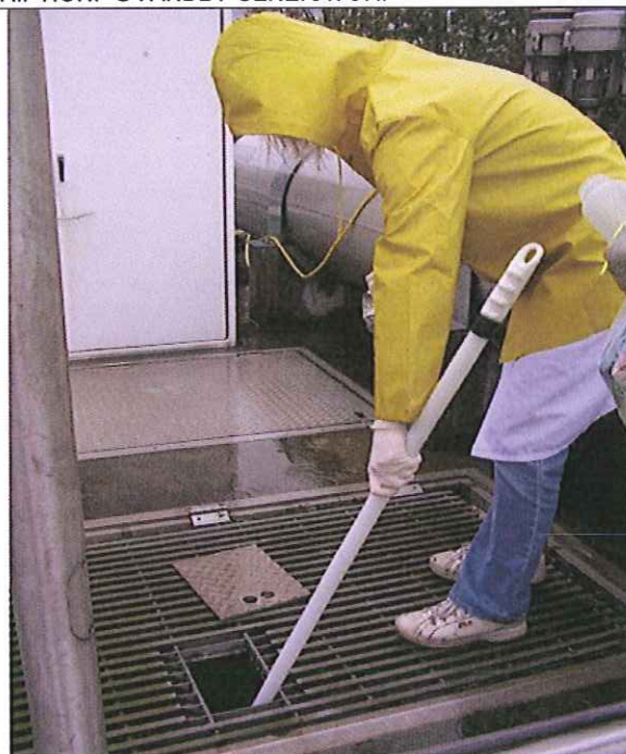
PHOTO #:16 DATE: 02/21/2012 TAKEN BY: MONIKA KANNADAGULI DESCRIPTION: EFFLUENT GRAB SAMPLE FOR FECAL COLIFORM ANALYSIS.
