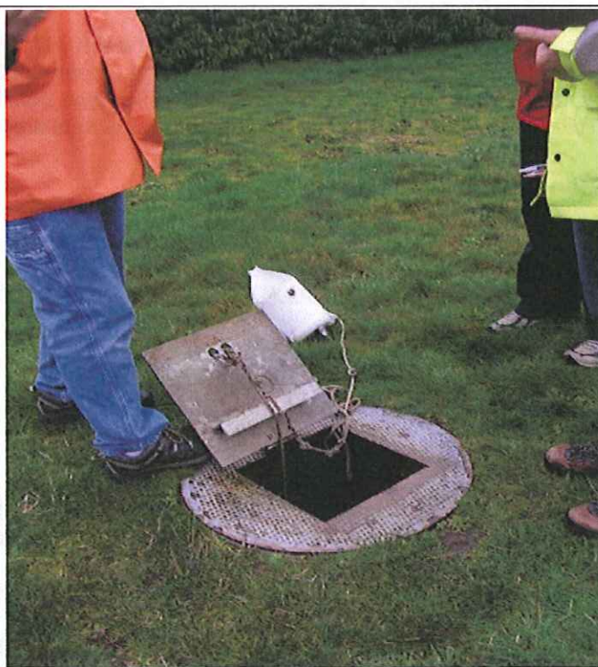
PHOTO #:02 DATE: 02/21/2012 TAKEN BY: MONIKA KANNADAGULI DESCRIPTION: INFLUENT GRAB SAMPLE FOR PROCESS CONTROL SAMPLES.
