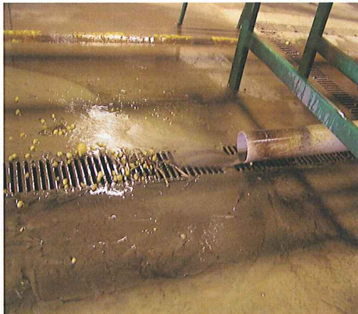
PHOTO #:06 DATE: 10/24/13 TAKEN BY: JEANNE TRAN DESCRIPTION: SCREENED WASH WATER IS THEN DISCHARGED INTO FLOOR SUMPS FOR COLLECTION AND SEDIMENTATION TREATMENT PRIOR TO BEING REUSED FOR SECOND AND THIRD WASHES. WASH WATER IS REUSED THREE TIMES PRIOR TO DISCHARGE TO THE SETTLING POND LOCATED NORTH OF THE FACILITY.
