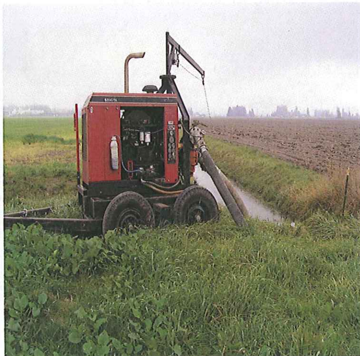
PHOTO #:19 DATE: 10/24/13 TAKEN BY: JEANNE TRAN DESCRIPTION: WATER FROM THE TRANSFER PIPE DISCHARGES INTO THE FIELD DITCH PRIOR TO BEING LAND APPLIED TO THE FIELD.
