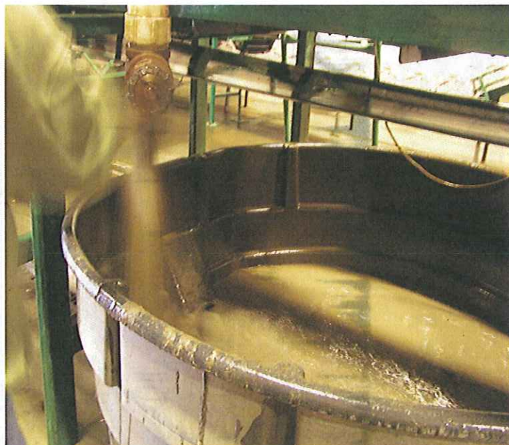
PHOTO #:05 DATE: 10/24/13 TAKEN BY: JEANNE TRAN: DESCRIPTION: WASH WATER BEING COLLECTED IN A LARGE TUB TO SCREEN OUT ROCKS AND LARGE DEBRIS.
