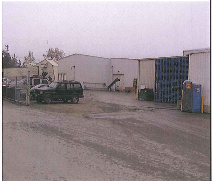
PHOTO #:010 DATE: 10/24/13 TAKEN BY: JEANNE TRAN DESCRIPTION: SOME AREAS OF THE PLANT ARE NOT PAVED, AND STORMWATER RUNOFF DRAINS INTO UNDERGROUND SUMPS, WHICH DRAIN INTO AN UNDERGROUND COLLECTION SUMP BEFORE IT IS GRAVITY DRAINED TO THE SETTLING POND.
