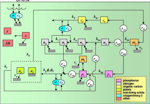
Figure 14. Kinetic Formulations for Simulating Dissolved Oxygen and pH in the Water Column Used by QUAL2K
