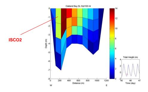
Figure 14. HOBO simulated maximum dye concentrations across the Oakland Bay sanitary line from run 15. Note that the ISCO2 sampler is positioned west of the peak concentrations, although it is closer to the outfall than the sanitary line being modeled (see Fig. 1).
