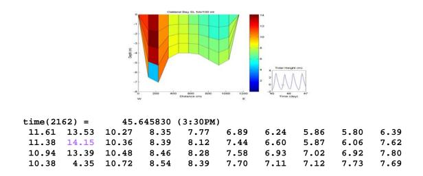
Figure 15. Fecal bacteria counts (# organisms per 100 ml) per cell for run 6 (4.0 mgd for 13 hours; ebb then flood with extended diffuser). This is the time step containing the peak concentration for the Oakland Bay sanitary line during this simulation.
