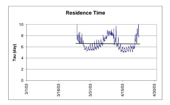
Figure 12. The calculated net-flow residence times from HOBO output across Hammersley Inlet (I=58). Results are for below the depth-of-no-motion using a 24.8-h moving average. The trend line is a linear best fit.
