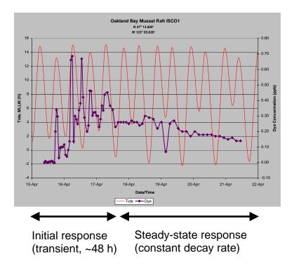
Figure 8. Time series of measured dye concentration at the Oakland Bay mussel raft (Fig. 1) on 15 Apr 2004. The concentration of effluent (bold) during the initial response phase of release is highly dependent on the initial conditions of the tide (light). During the steady-state phase, the response exhibits first-order (exponential) decay.
