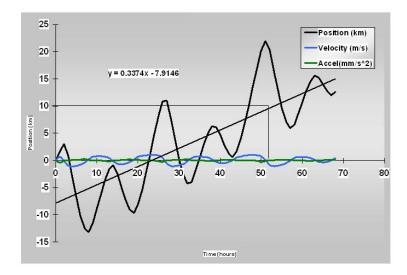
Figure 10. Approximate solution for a perfect channel with friction. f = 0.025 N-s/m (kg/s), h = 6.8 m, dx (distance between gauges) = 8.1488 km).
