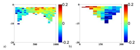
Figure 11. Residual flow as calculated by averaging eight ADCP transects on 16 April 2003 across a) Oakland Bay and b) Hammersley Inlet.
