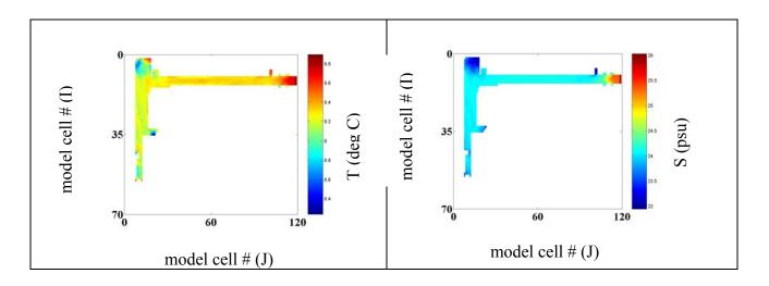
Figure 5. Surface-layer temperature and salinity on computational plane prior to adding tides in HOBO.
