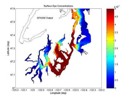
Figure 16. Apparent fate and transport of Oakland Bay effluent seaward according to the South Puget Sound Synthesis Area Model.
