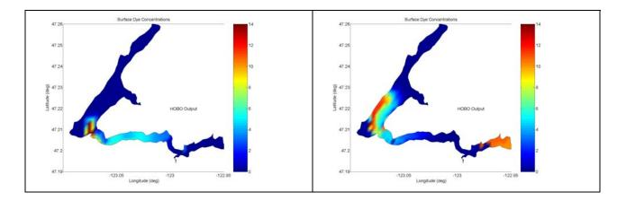
Figure 13. Plan view of the adverse condition (ebb tide after flood) for the Oakland Bay sanitary line from HOBO run approximating actual dye-release conditions (run 15): a) time = 45.479 days, b) time = 45.531 days.
