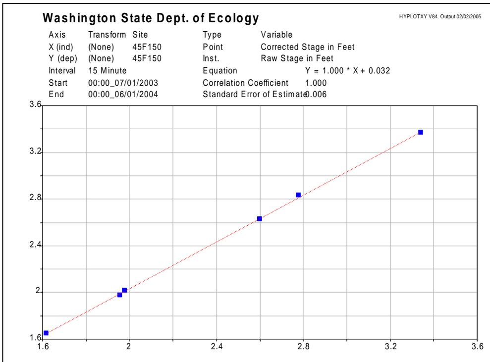
Figure 43: Linear regression of staff gage versus pressure transducer readings for Site 13.
