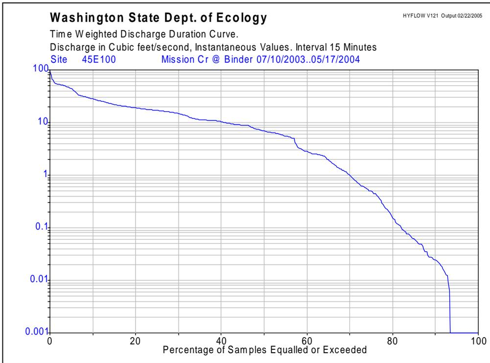
**Figure 30: Discharge exceedence graph for Site 10.**
