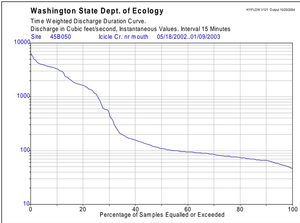
Figure 4: Discharge exceedence graph for Site 1.
