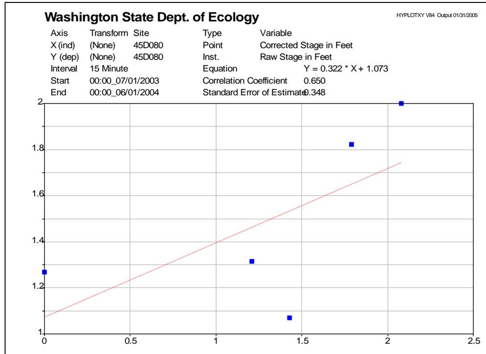
Figure 35: Linear regression of staff gage versus pressure transducer readings for Site 11.
