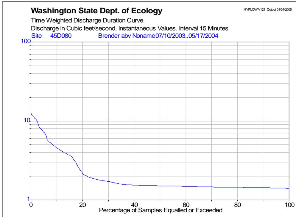
Figure 34: Discharge exceedence graph for Site 11.
