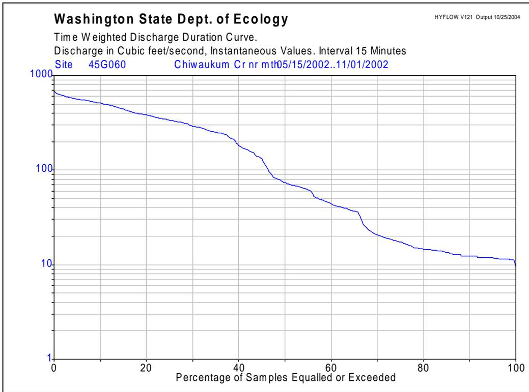
**Figure 8: Discharge exceedence graph for Site 2.**
