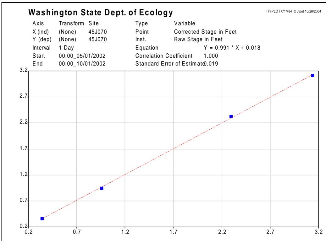
Figure 13: Linear regression of staff gage versus pressure transducer readings for Site 3.
