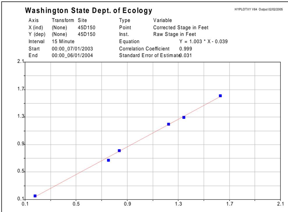
**Figure 39: Linear regression of staff gage versus pressure transducer readings for Site 12.**
