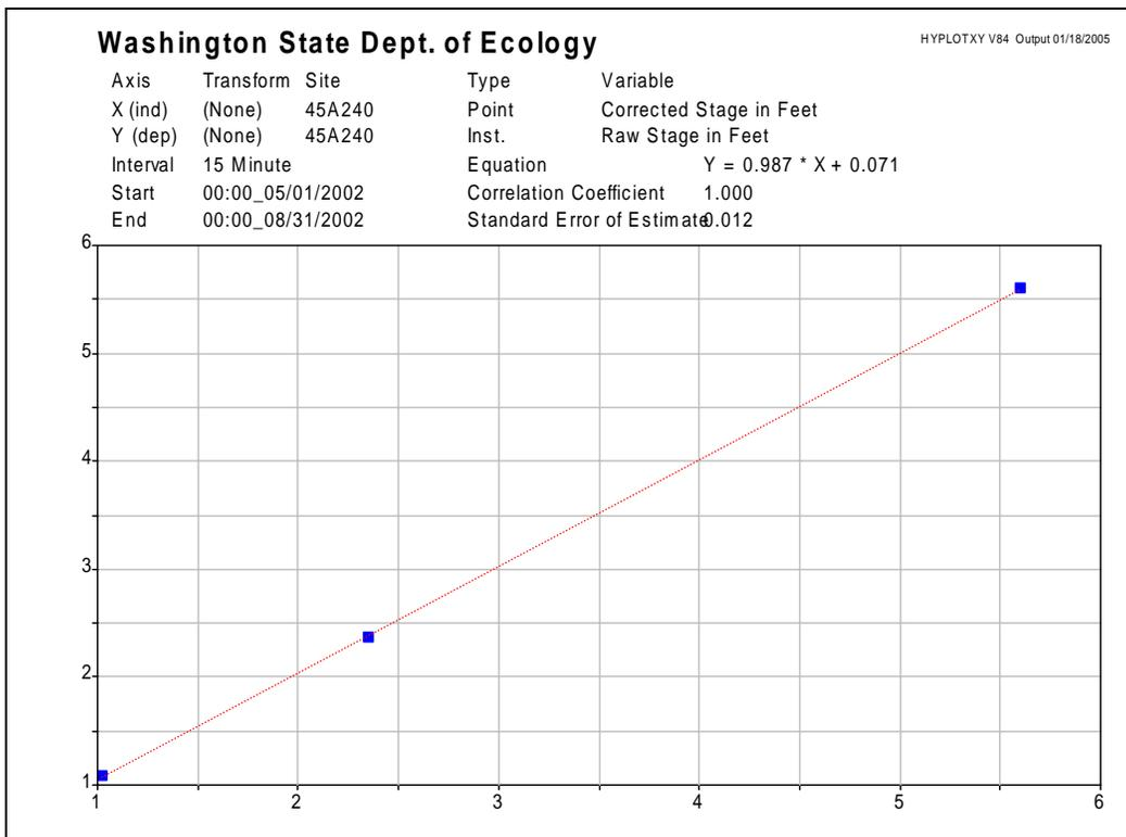
**Figure 17: Linear regression of staff gage versus pressure transducer readings for Site 4.**
