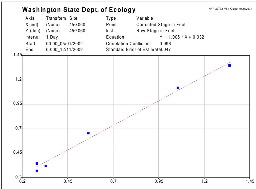
**Figure 9: Linear regression of staff gage versus pressure transducer readings for Site 2.**
