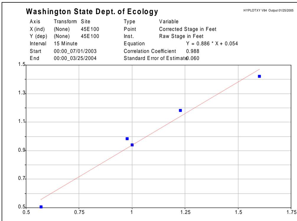
**Figure 31: Linear regression of staff gage versus pressure transducer readings for Site 10.**
