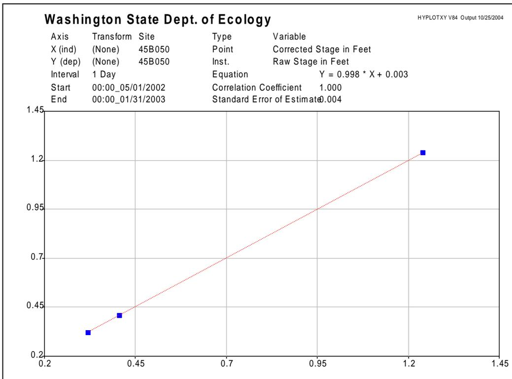
Figure 5: Linear regression of staff gage versus pressure transducer readings for Site 1.
