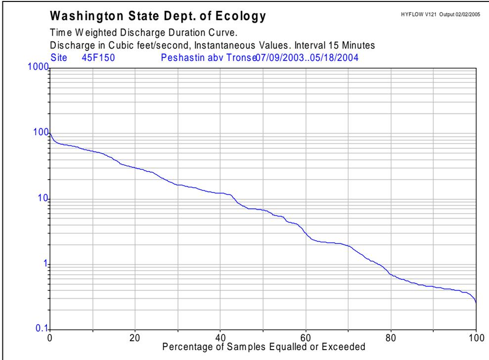
Figure 42: Discharge exceedence graph for Site 13.
