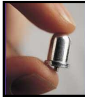
Figure 1: This small automotive light switch contains one gram of liquid mercury.
