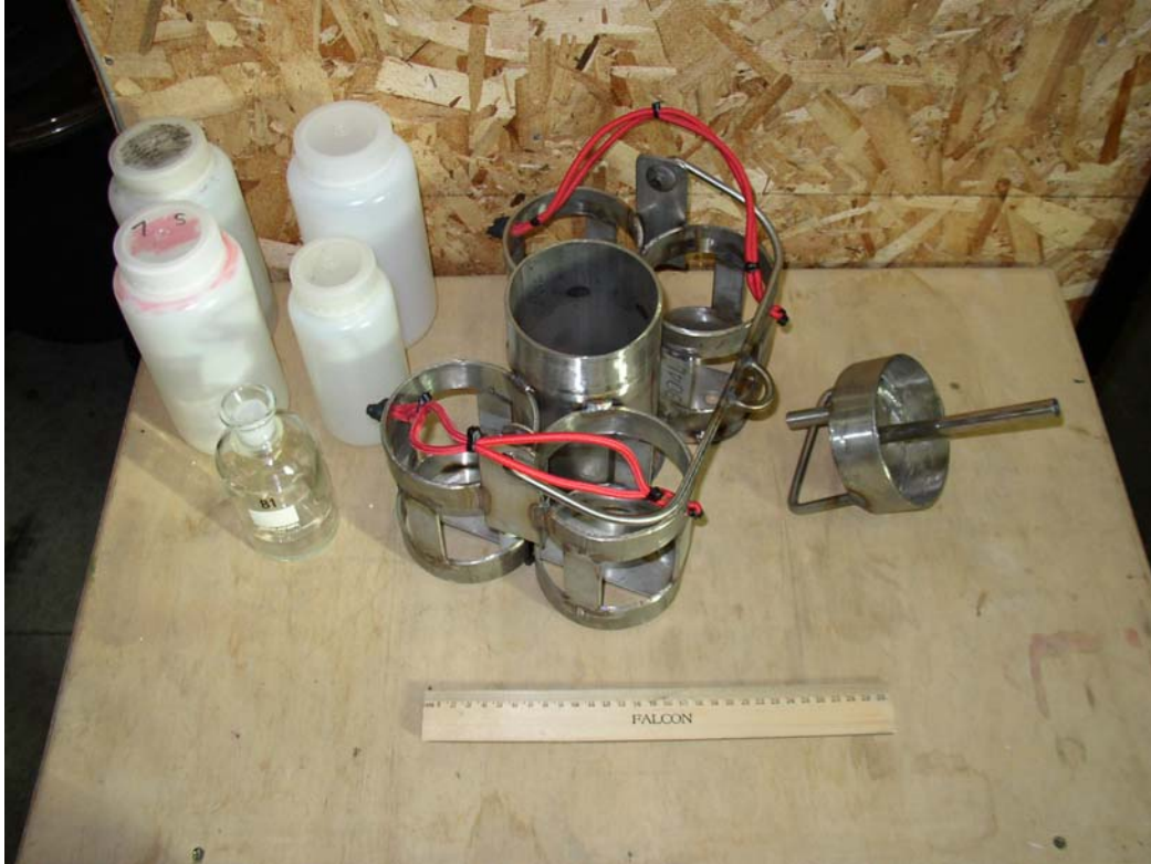
Figure 1. Our new sampling device (designed by Bill Ward). Oxygen is collected in the bucket; all other samples are collected in passengers.
