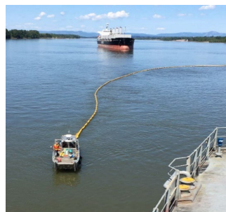
Unique pre-booming configuration used on the Columbia River. This configuration accounts for river current.
