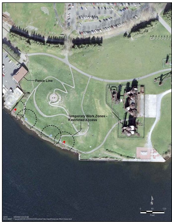
Photo at left showing western shoreline of Gas Works Park with drilling locations and areas to be closed to public access during drilling activities.
