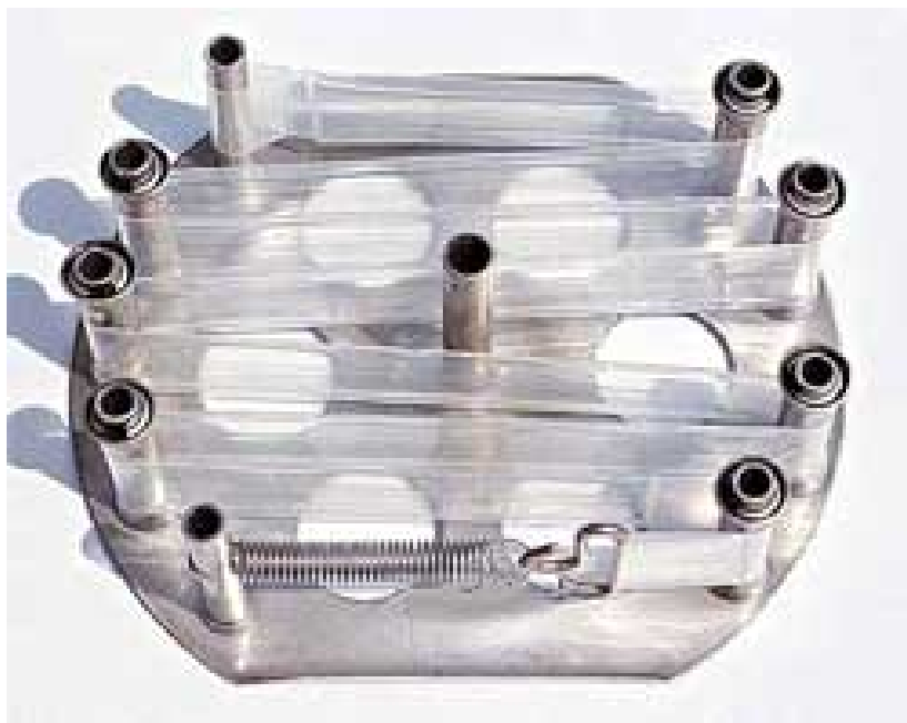
Figure 1. Standard SPMD Membrane Mounted on a Spider Carrier.
