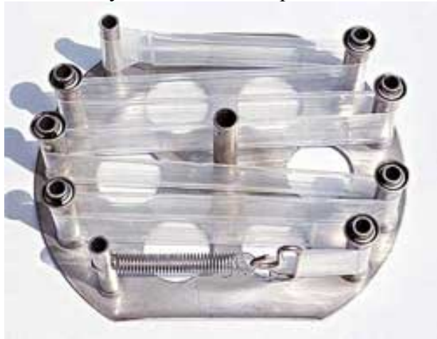
Figure 6. Standard SPMD Membrane Mounted on a Spider Carrier.
