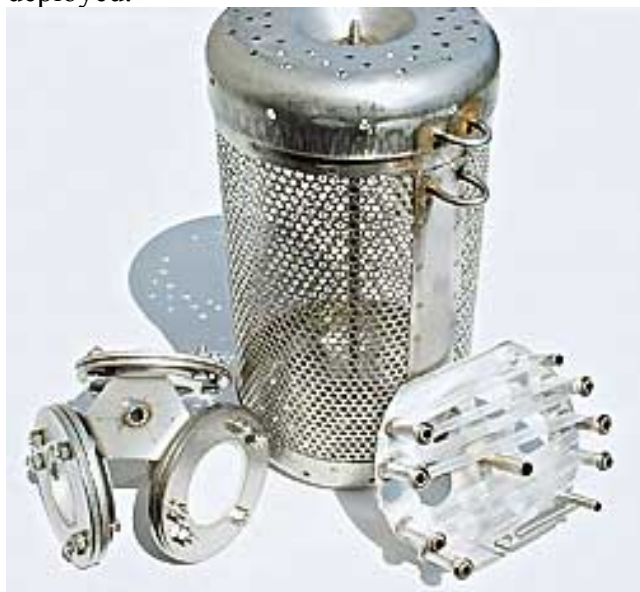
Figure 8. Large canister which may fit six POCIS membranes (two per carrier on left) or five SPMDs (right).
