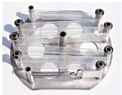
Figure 2. Standard SPMD membrane mounted on a spider carrier.
