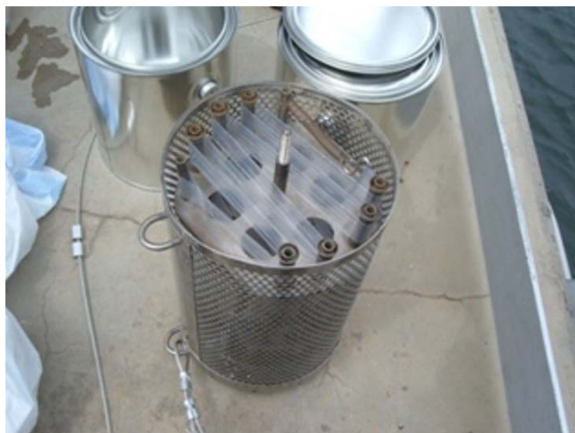
Figure 3. SPMDs Mounted on Carriers Inside a 5-membrane Canister. Shipping Cans in Background.
