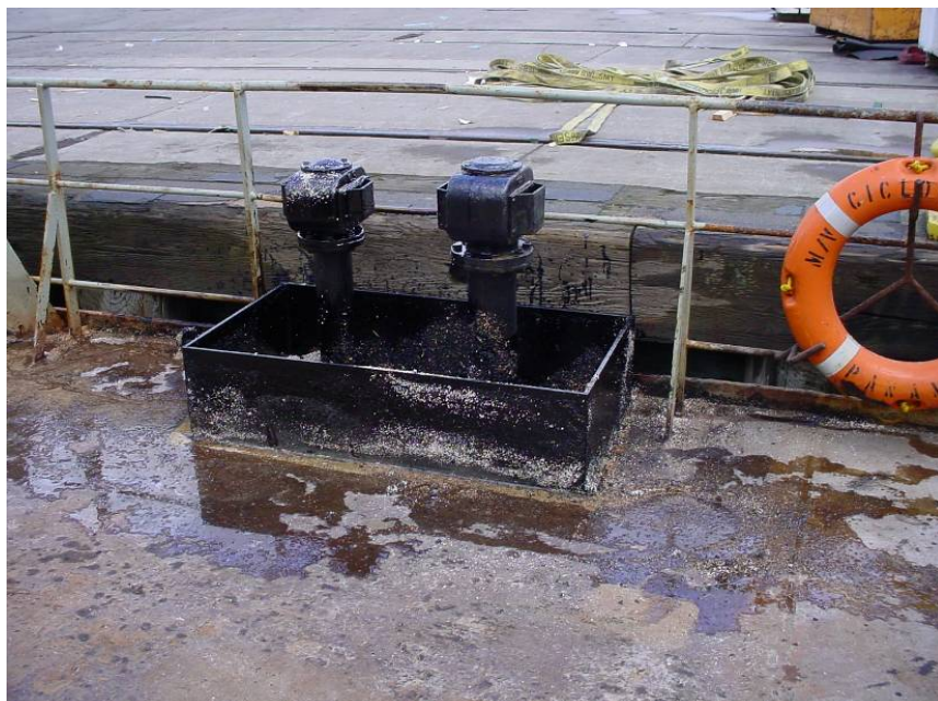
Figure 3 - No. 1 starboard fuel oil tank vents from which oil spilled. Note: Oil splattering on pier.
