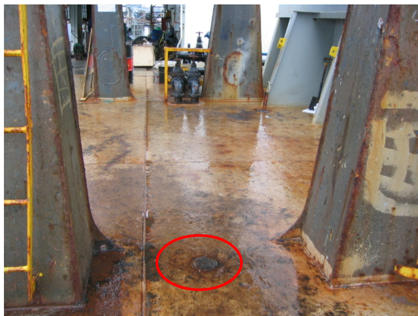
Figure 4 - Location of recessed starboard sounding tube cap (view looking aft toward starboard fuel oil header).
