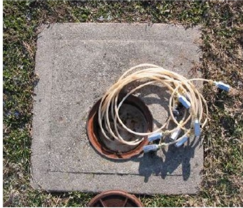
Figure D-5: Photograph of permanent multi-depth nested soil gas sampling probes using small diameter tubing. (Credit: H&P Mobile Geochemistry)
