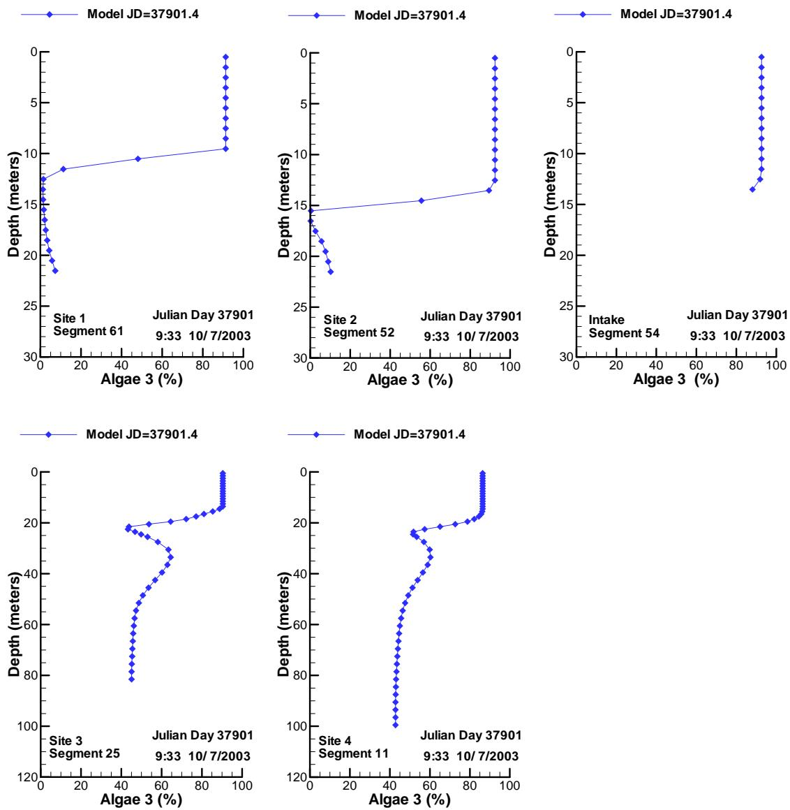
**Figure 710.** Vertical profiles of CYANOBACTERIA compared with data for 10/7/2003.
