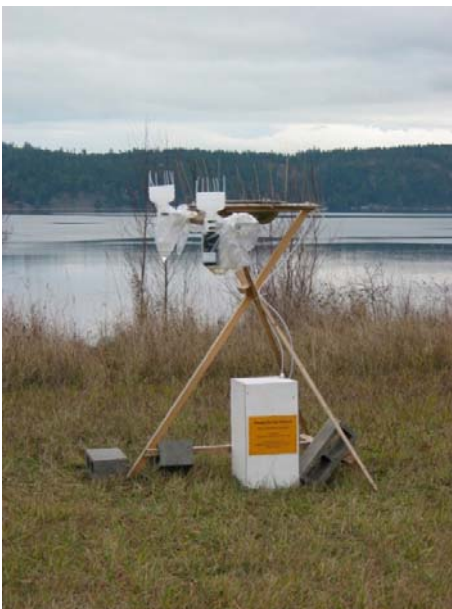
Figure 2. Bulk atmospheric deposition collector with stainless steel funnel in the center draining down into the wood box for organic parameters, clear Teflon ® 1L bottles for trace elements (left arm), and opaque Teflon ® 1L bottles for mercury speciation (right arm).
