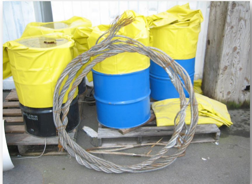
Broken tow wire section from an incident involving a drifting tank barge.
