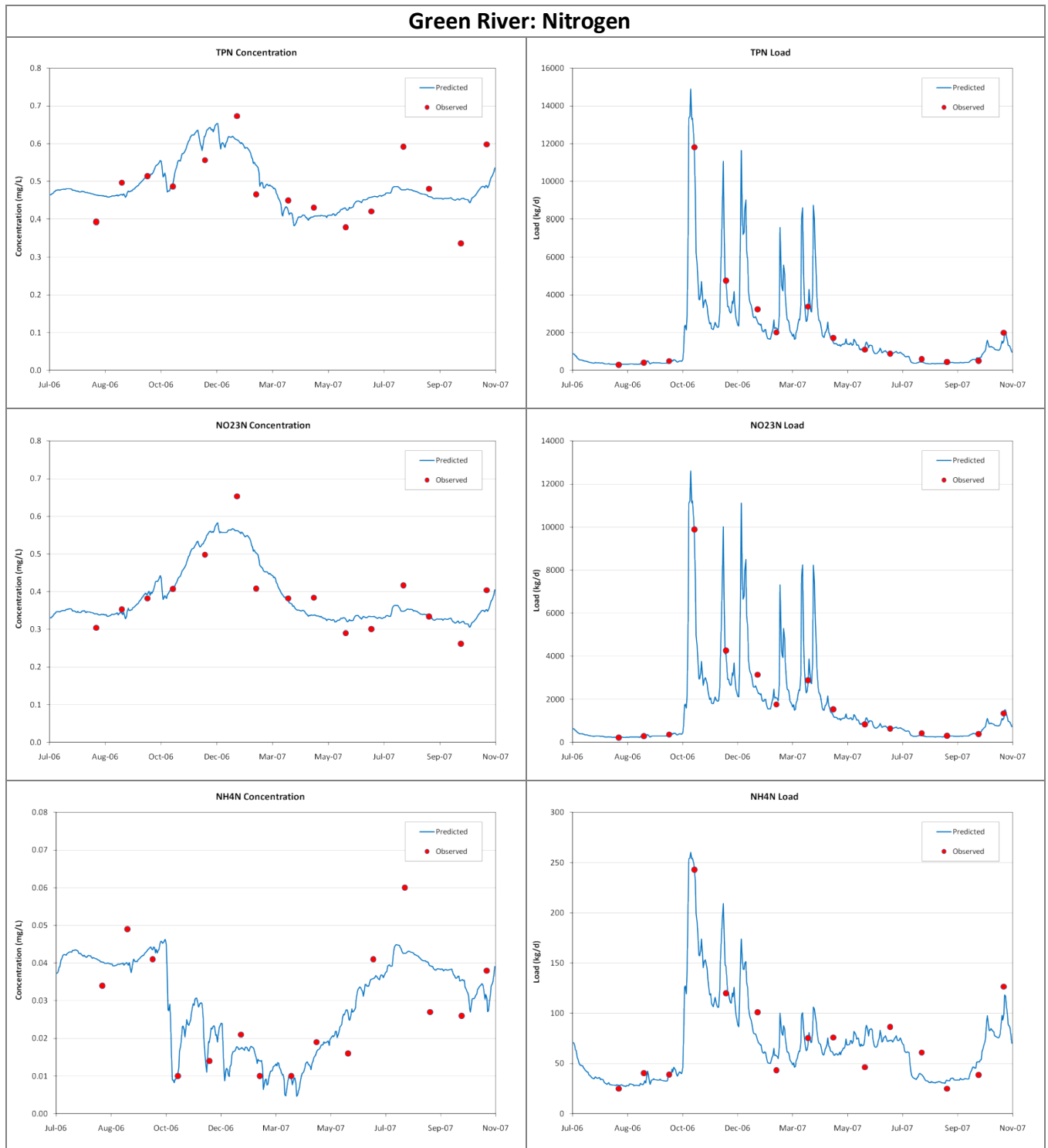
Figure D-4. Predicted and observed concentrations (left column) and loads (right column) of nitrogen for the Green River.
