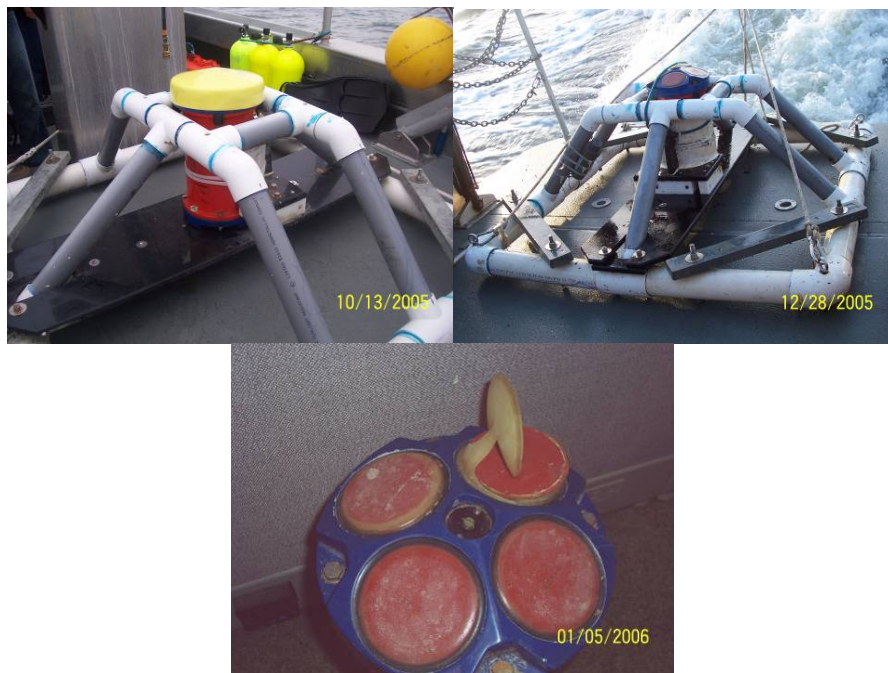
Figure G-7. ADCP before deployment (left), after retrieval (middle), and close up of exploded lens (right).
