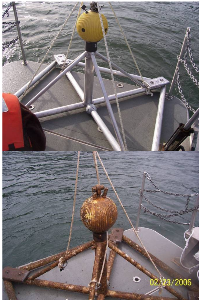
Figure G-5. InterOcean S4 device before deployment (left) and upon retrieval (right).
