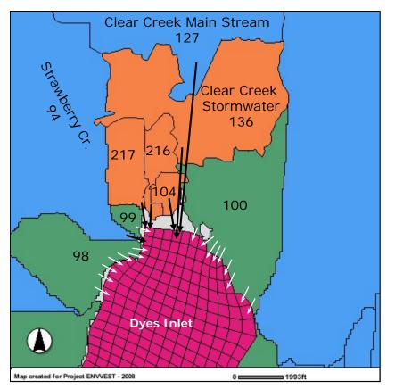
**Figure 8. Linkage between flows from watershed and marine grid cells (red).** *Flows from streams (blue watersheds) and stormwater outfalls (orange watersheds) shown by black arrows, and shoreline drainages (green watersheds) shown by white arrows. Numbers are the DSNs used n the model.*
