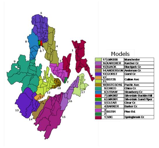
Figure E1. Delineated watersheds, landscape segments, and HSPF sub-basin models used to model hydrologic runoff from the Sinclair and Dyes Inlets watershed.
