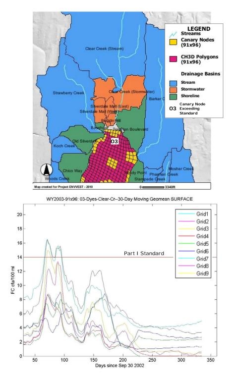
Figure 15. Canary node 03-Dyes-Clear-Cr at northern Dyes Inlet *(upper figure)* and simulated 30-day moving geomean for the nine grid cells (lower) from "Actual Conditions" model run.
