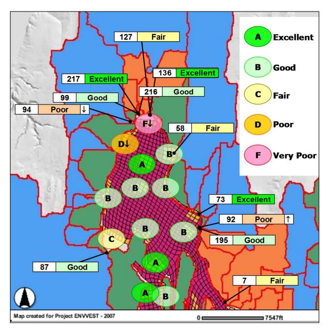
Figure E11. Model evaluation results for estimating FC loading from watershed DSNs (rectangles) and predicting FC concentrations at canary nodes (circles) in Dyes Inlets during WY2003 (from Figure 4-46 in Johnston et al., 2009) Arrow pointing up means over-prediction; arrow pointing down means underprediction of FC concentration.
