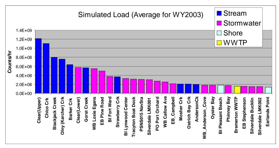
Figure 12. Simulated average yearly loads (counts/hr) for the top 30 sources of FC discharges into Sinclair and Dyes Inlets based on modeled hourly loads over the year.
