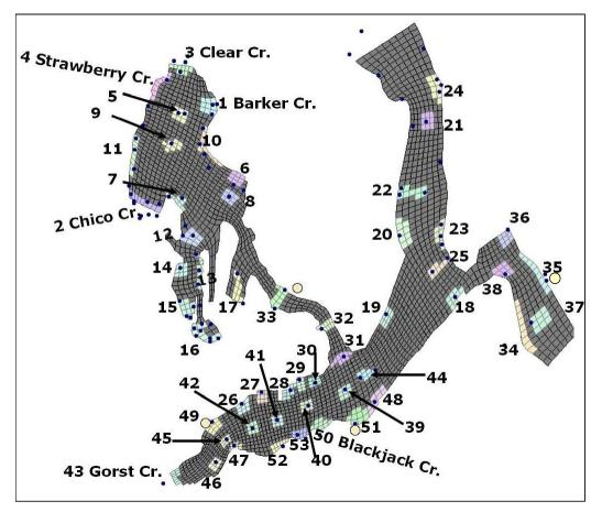
Figure 9. "Canary nodes" (numbered groups of nine marine grid cells) were selected based on proximity to known pollution sources. *Monitoring sites are blue dots and WWTP discharge locations are yellow circles.*
