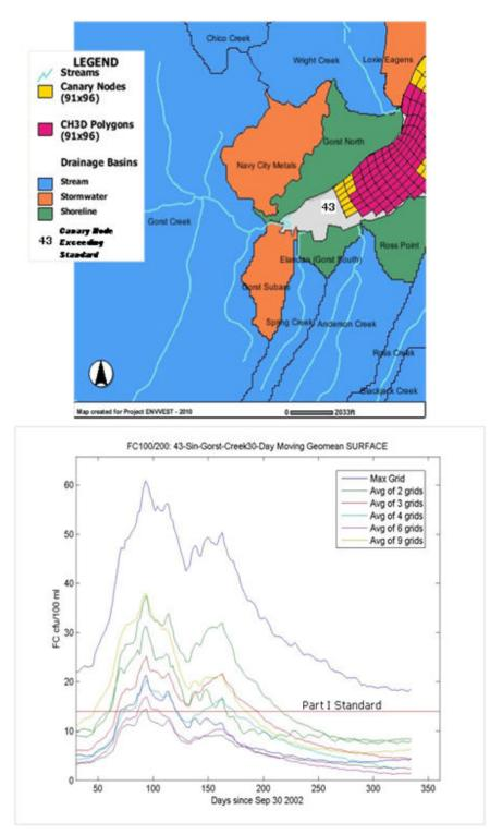
**Figure 16.** Location of canary node for receiving waters below Gorst (upper figure). Simulated 30-day moving geomean for surface grid cells of the Gorst canary node from WY2003 100/200 model run (lower figure).
