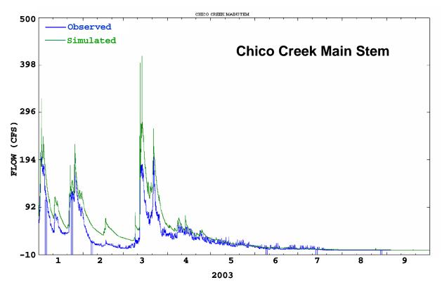
Figure E3. Results of HSPF model verification of Chico Creek main stem for observed (blue) and simulated (green) flow for 2003 (from Figure 2-7 in Johnston et al., 2009)
