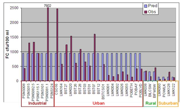
Figure E6. Predicted (Pred) and observed (Obs) FC geomean concentrations for industrial, urban, rural, and suburban stormwater outfalls in watershed (from Figure 2-13 in Johnston et al., 2009).
