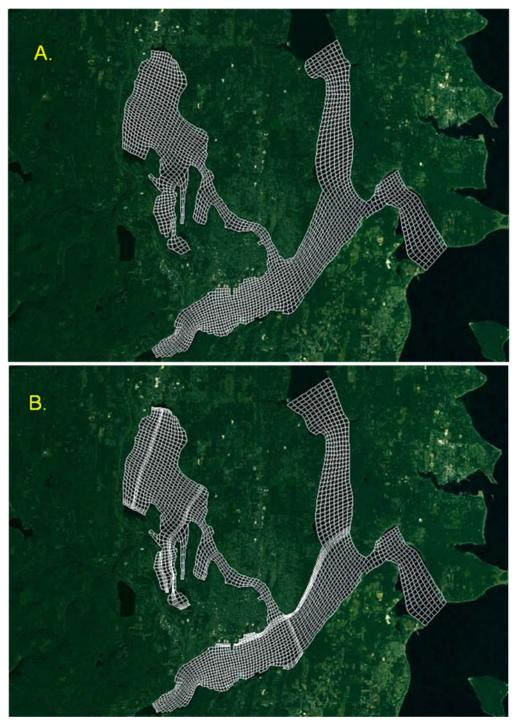
Figure E8. The computational grids used for CH3D-FC including the 91 x 96 grid (A) and the 94 x 105 grid (B) that has higher resolution in nearshore areas.
