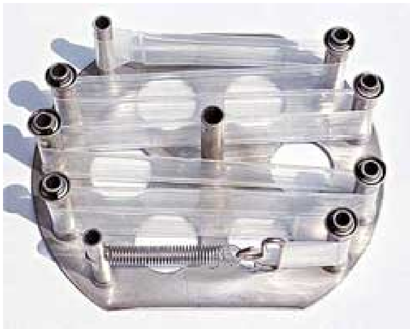
Figure 2. Standard SPMD Membrane Mounted on a Stainless Steel Spider Carrier.
