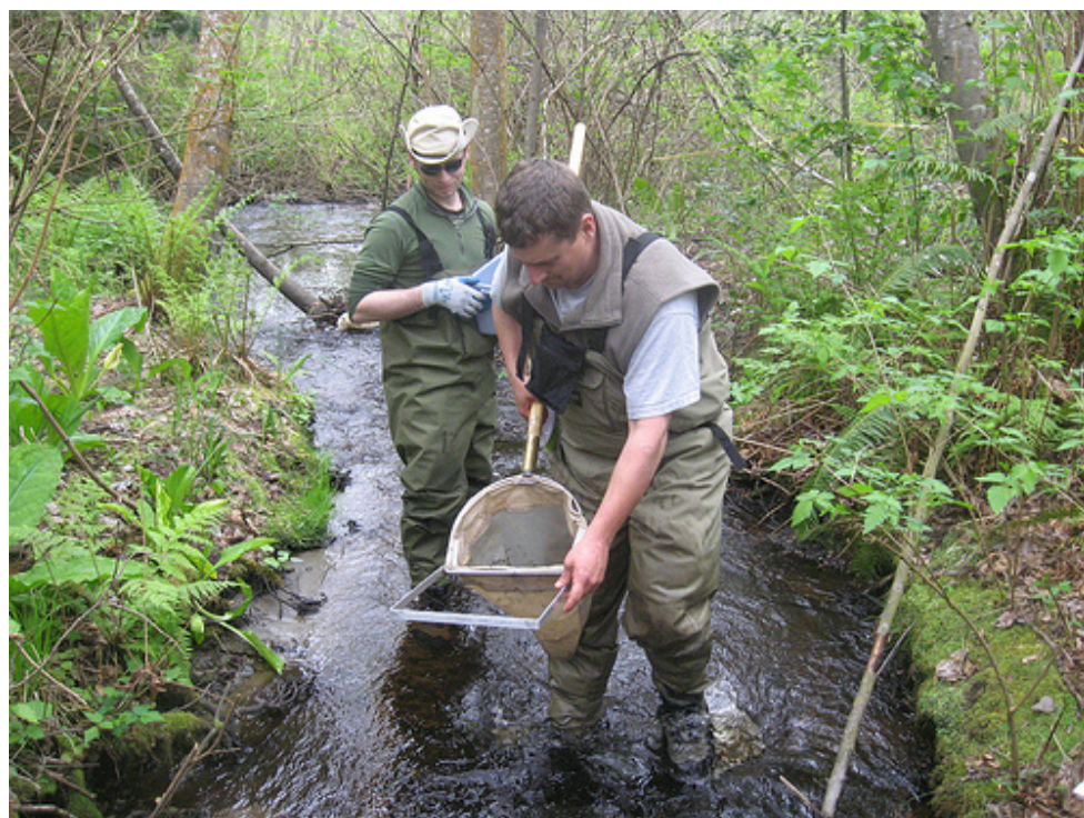
Figure C-3. Benthic Macroinvertebrate Collection using a D-Frame Kicknet.
