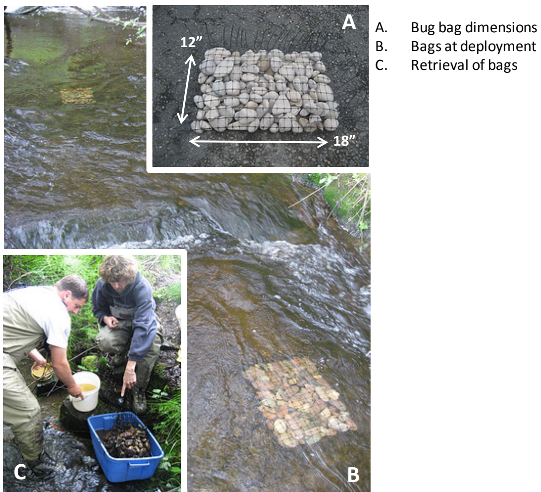
Figure C-4. Bug Bag Method of Benthic Macroinvertebrate Collection.
