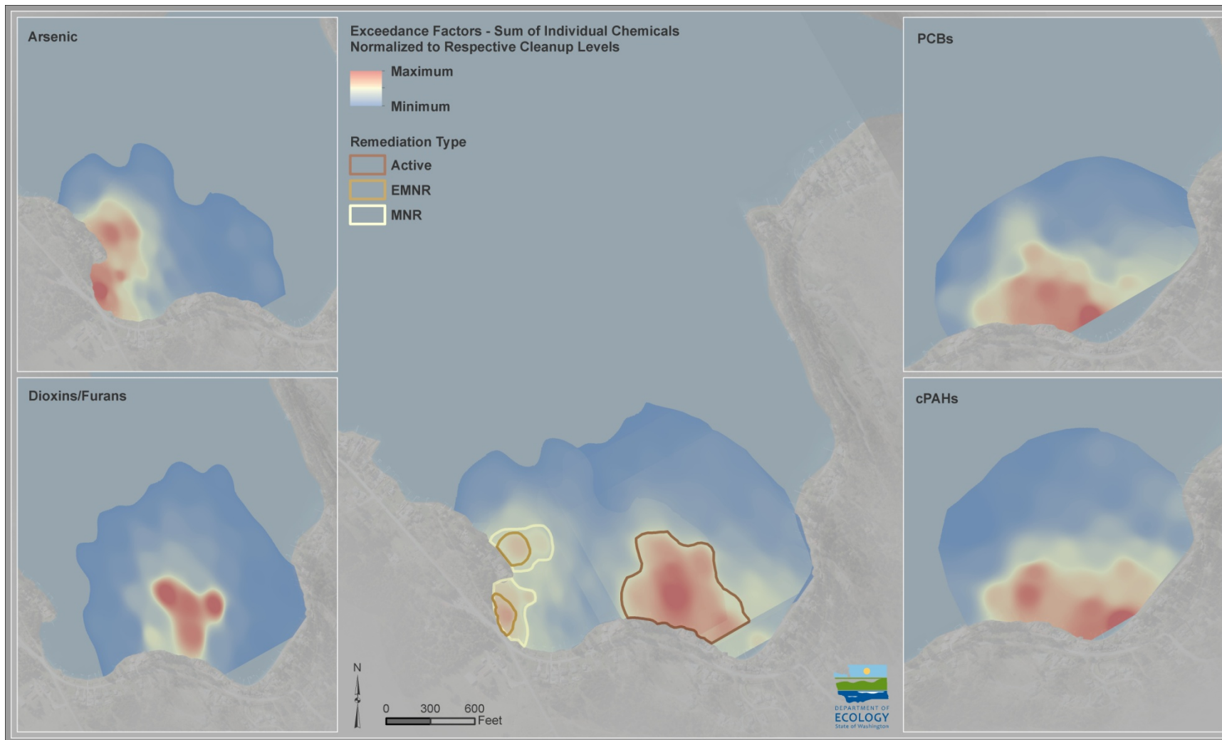
Figure 6-10. Complex site with overlapping CoCs normalized to cleanup levels (“exceedance factors”), summed to portray areas of highest concern.
