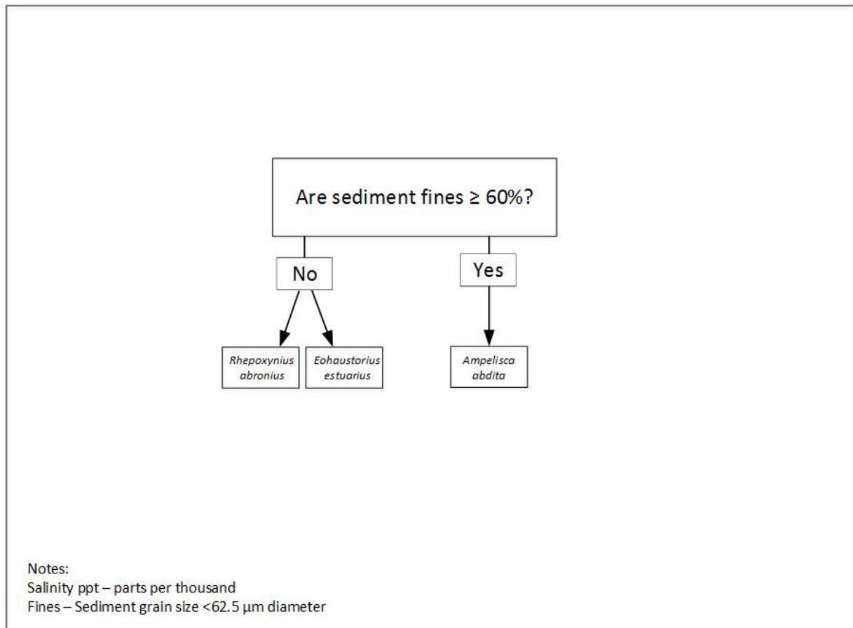
Figure 4-1. Selection of appropriate amphipod species for marine/estuarine toxicity tests.
