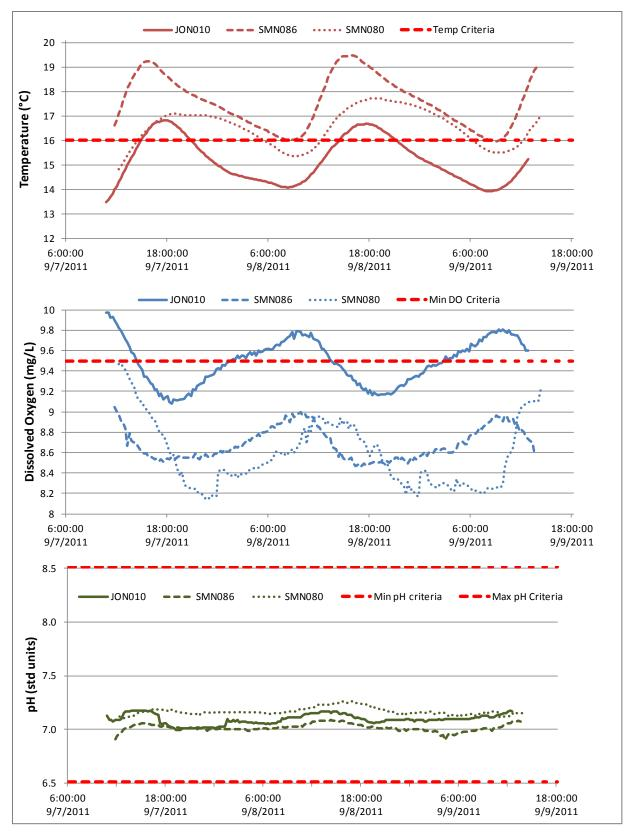
Figure 10. Continuous water quality data for Upper Salmon Creek sites and Jones Creek collected during the additional deployment in early September 2011.
