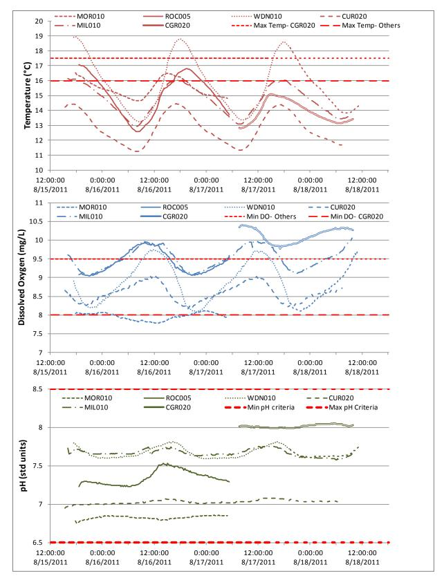
Figure 9. Continuous water quality data for Salmon Creek tributary sites collected during the August synoptic survey.
