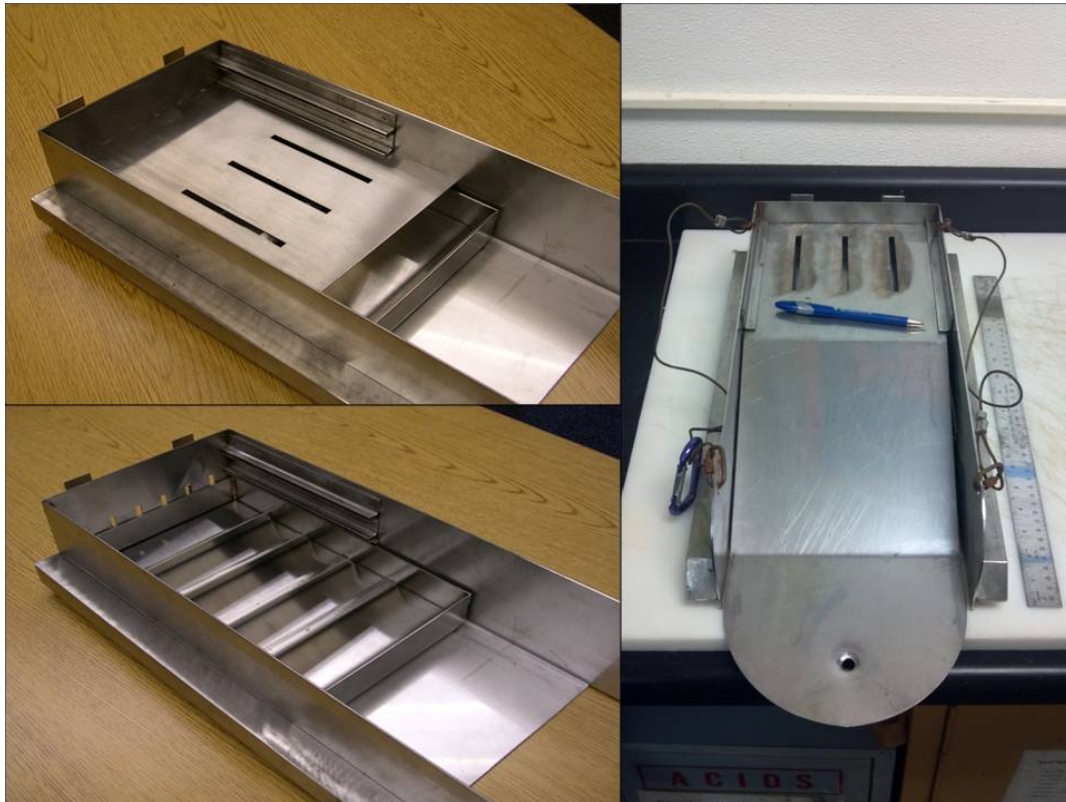
Figure 4. Hamlin Sediment Trap Used to Collect Suspended Sediments.
