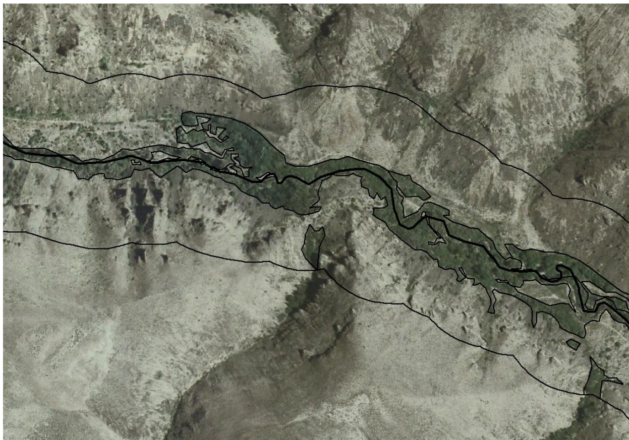
Figure 11. Example of a color digital orthophoto showing digitized riparian vegetation.
