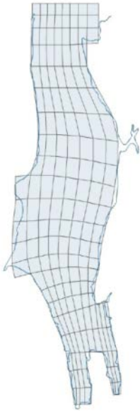
Figure 4. GEMSS model grid used for calibration of the Budd Inlet model.
