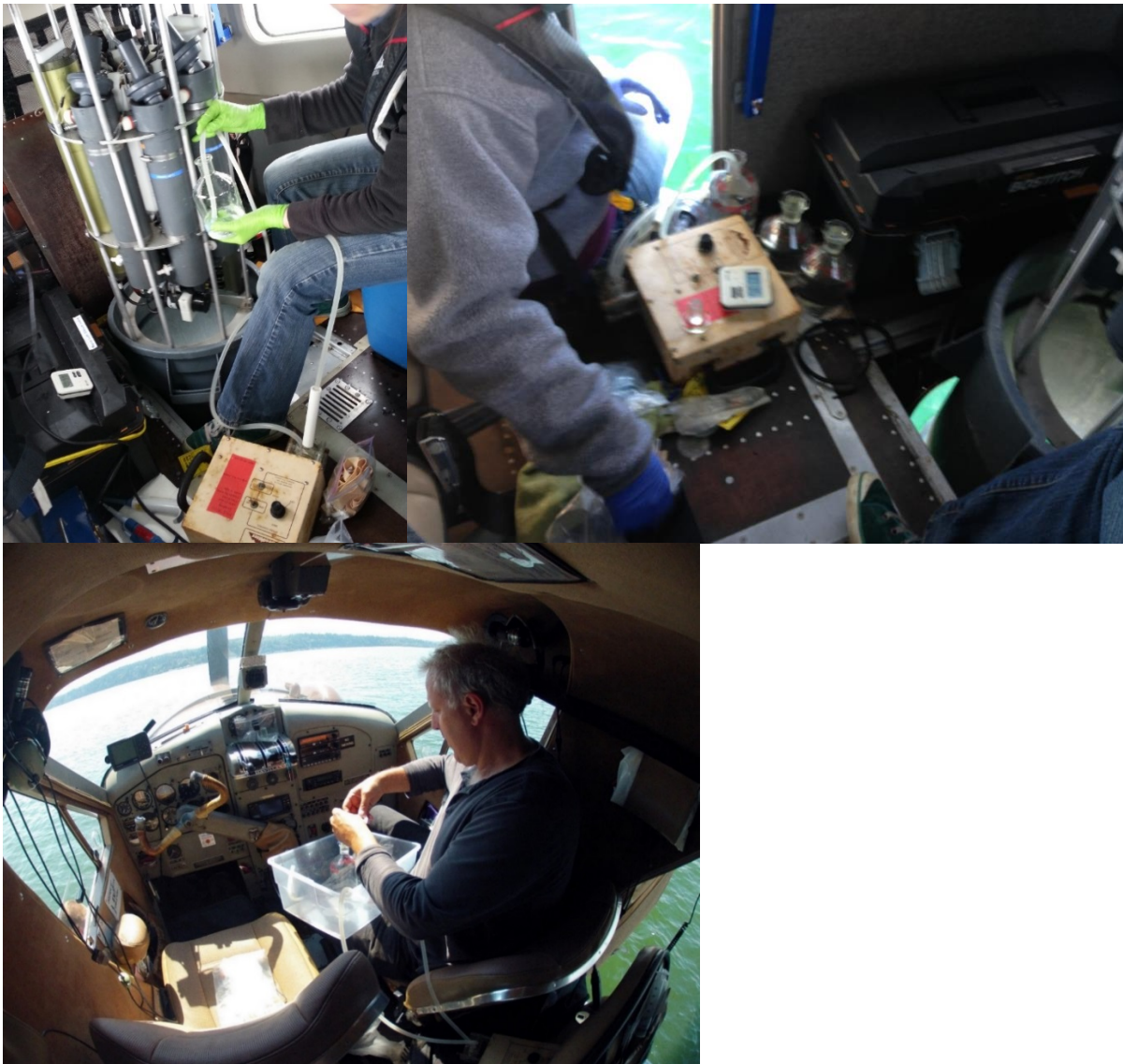
Figure 2. Three versions of TA/DIC sampling setups in the floatplane.
