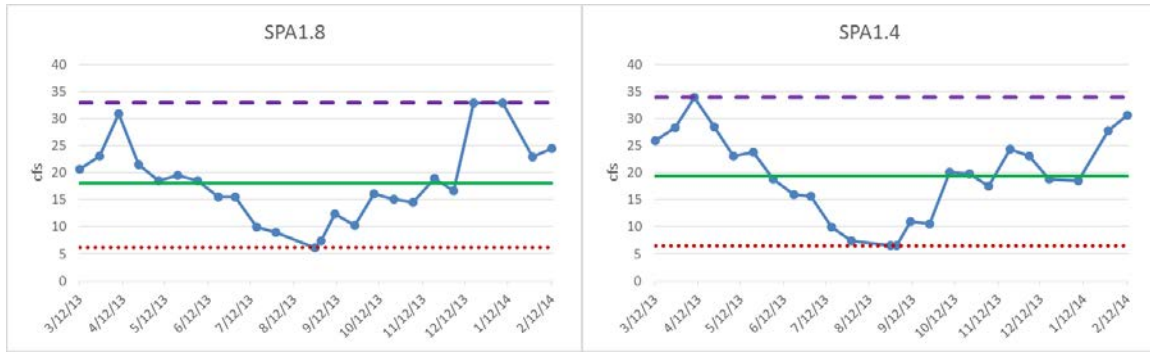
Figure A-28. Instantaneous discharge measurements by Ecology from March 2013 to February 2014. Horizontal lines show minimum, mean, and maximum values from bottom to top.
