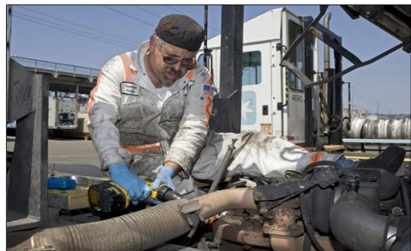
**Photo 25:** Retrofitting an engine to reduce emissions. Photo credit: Ecology
