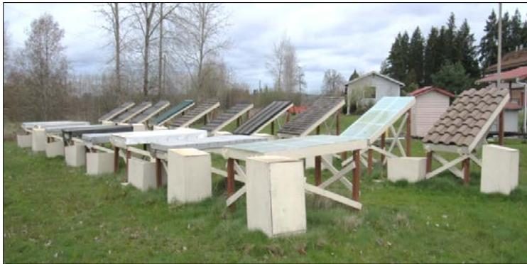
**Photo 22:** Roofing panels were evaluated for potential leaching of metals and organic chemicals during storm events. Photo credit: Washington Stormwater Center (WSC)
