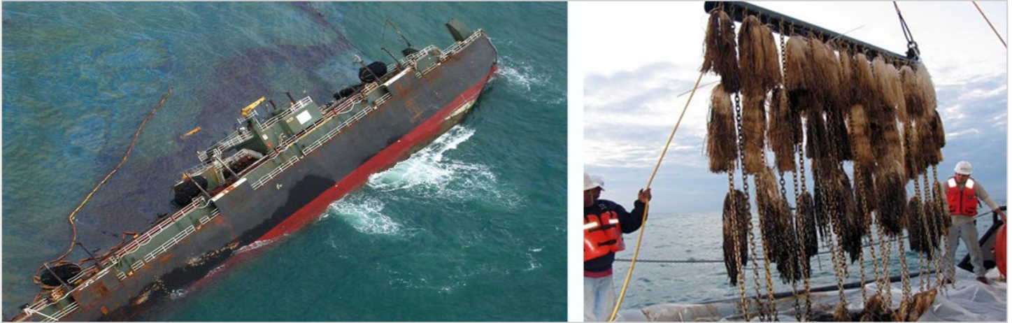
The 2005 tank barge DBL 152 incident (left) spilled 1.9 million gallons of heavy oil, most of which sank to the bottom of the Gulf of Mexico. Oil absorbent material attached to chains (right) was dragged on the seafloor, which is one method for detecting submerged oil. (Credit: NOAA)
