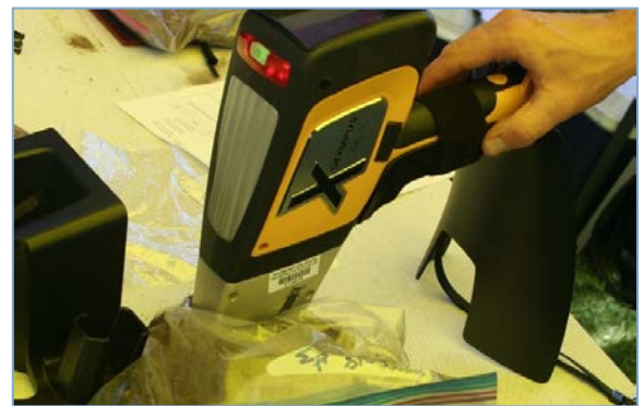
Photo 9: At the soilSHOP on Vashon Island soil is screened for lead and arsenic contamination by staff using an X-ray fluorescence (XRF).
