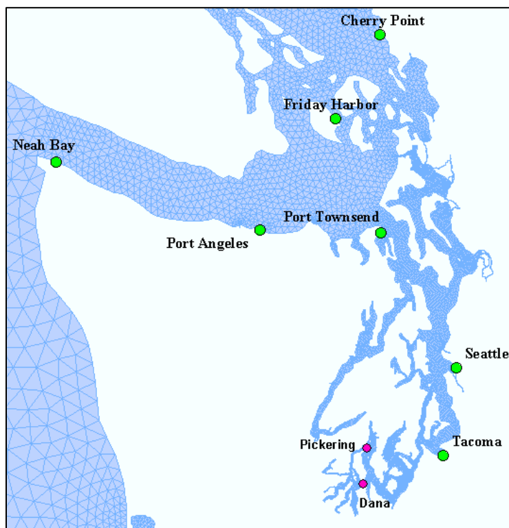
Figure 10. National Oceanic and Atmospheric Administration (NOAA) stations (green dots), where model-predicted water surface elevations were compared with observed data, and Acoustic Doppler Current Profiler (ADCP) stations (red dots), where model-predicted currents were compared with observed data.
