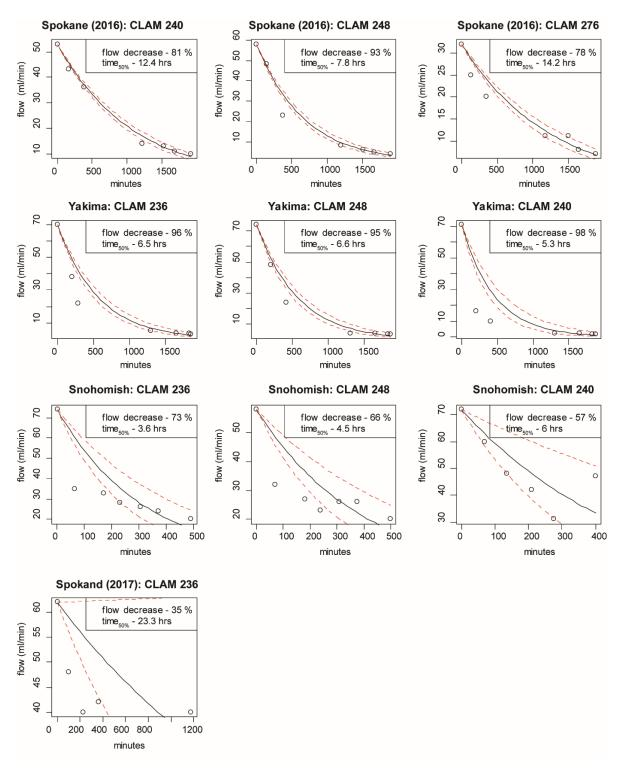
Figure A-1. Measured CLAM flow rates during deployment.
