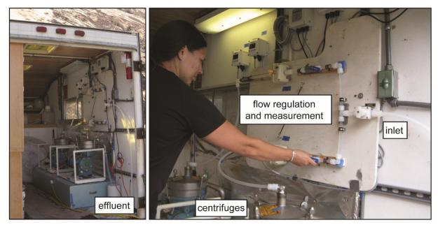
Figure 6. Centrifuge trailer (left) and the flow control board for each centrifuge (right).
