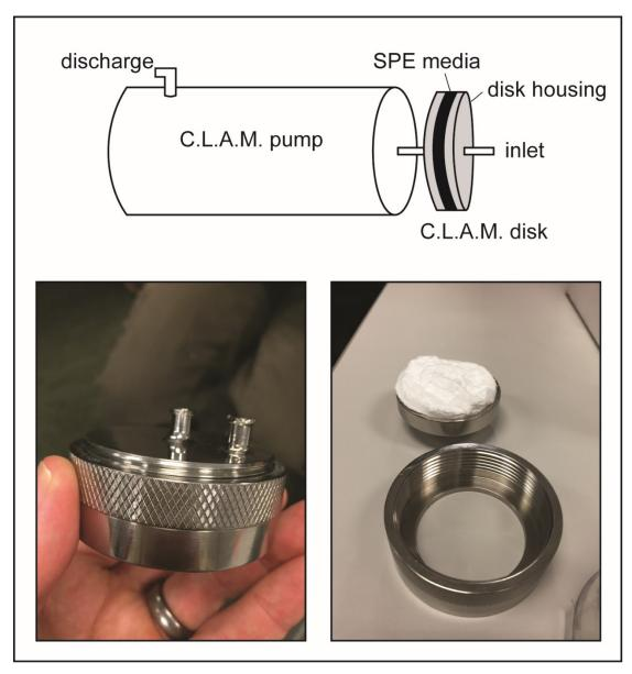
Figure 5. Parts of the CLAM sampler. Top: Schematic of the CLAM sampler showing the position of the disk. Bottom-right: Inside the disk housing; the white material is the SPE media. Bottom-left: Assembled stainless steel CLAM disk housing.
