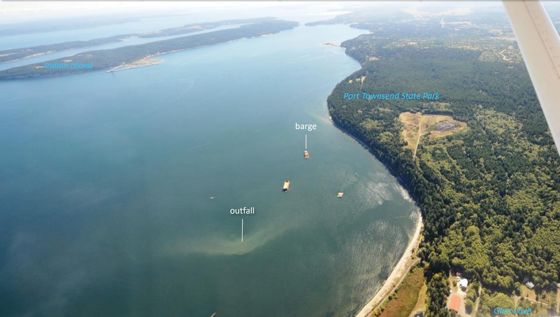
Water with surfacing turbidity, likely from an underwater diffuser. Location: Port Townsend Bay (North Sound), 1:25 PM
