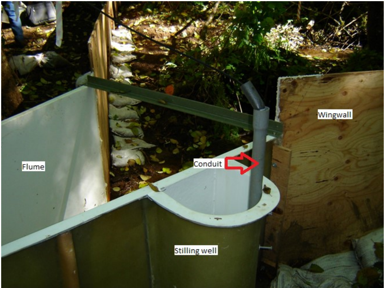
Figure 2. Pressure transducer and conduit in a Type N study stream. Cable ties secure the pressure transducer within the conduit. Holes drilled into the base of the conduit allow water exchange. Bolts secure the conduit to a stilling well and flume.
