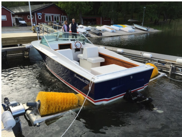
Figure 4 Picture of drive-in boatwash station at Bosö Boat Club, Stockholm N
