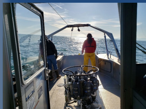
Above: I help collect water samples using a CTD Below: We also collect CTD data via float plane
