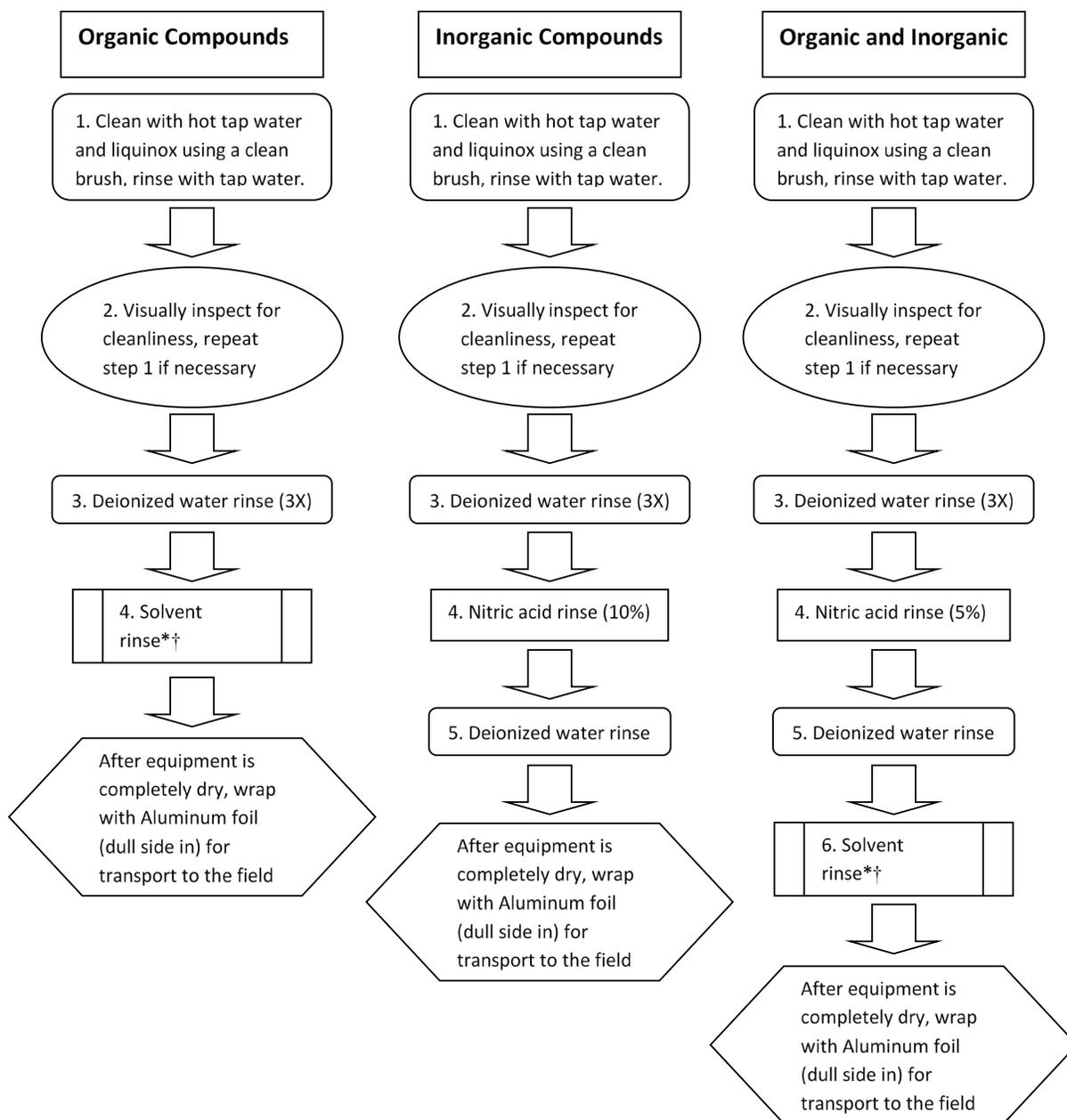
**Figure 1. General procedure for decontaminating equipment when sampling for organic or inorganic contaminants.**
