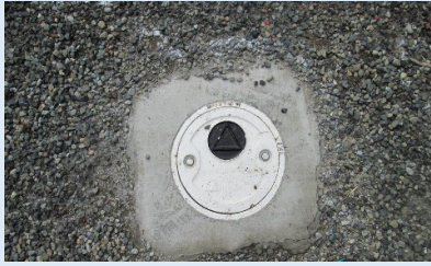
Figure 1. A monitoring well on the Boeing Auburn Site. Boeing will take samples from monitoring well access points to track the concentration of TCE on the site over time.
