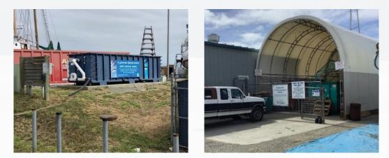
Centralized oil collection location. Putting all the oil collection and management devices in one location lessens the impact from oil sitewide and means that there is only one place to worry about when it comes to oil management.
