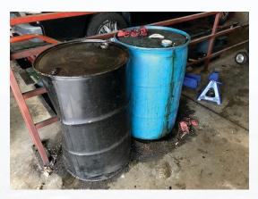
Before: The area lacked secondary containment. These drums were located next to stairs leading to the pit below. Spills in this area would be extra difficult to clean up.
