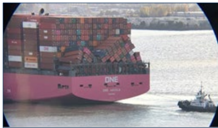
Figure 42: Remote visual monitoring by inspector Scott Wurster of the container ship ONE AQUILA inbound to Tacoma with collapsed containers
