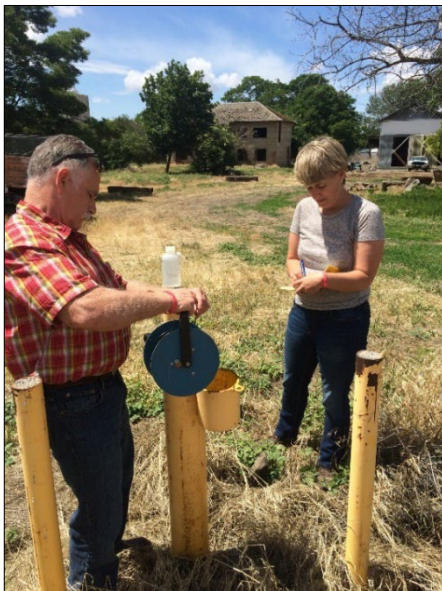
Figure 30: Ecology cleanup site managers Bill Fees and Sandra Treccani check the depth to groundwater in one of monitoring wells used to track cleanup progress at the Schwerin Concaves site in Walla Walla, Walla Walla County. Credit: Ecology, Cleanup Site ID 3956.
