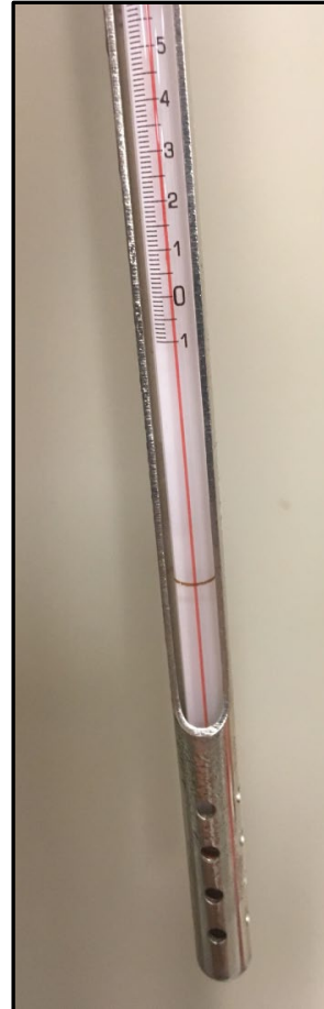
Figure 1. Left: A partial immersion alcohol (liquid in glass) thermometer immersed in water to the immersion line, below the incremental temperature marks on the stem and above the alcohol filled bulb. Photo by Dan Dugger.
