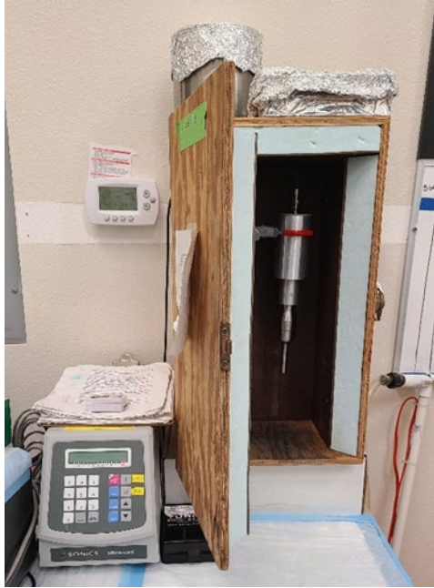
Figure 3. Sonicator control box and wooden insulated box where samples go.
