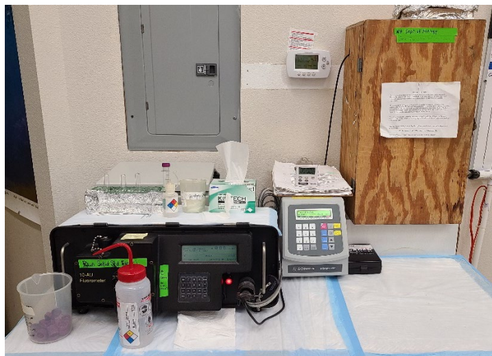
Figure 2. Benchtop Fluorometer with 90% acetone bottle, cap beaker, vial rack, kimwipes, and sonicator.
