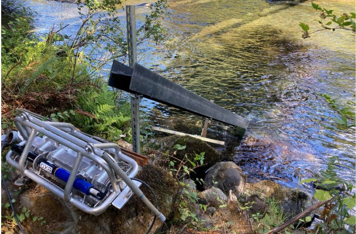
Figure 2. Probe shuttle and I-beam test deployment at the South Fork Newaukum River at Jorgenson Road.
