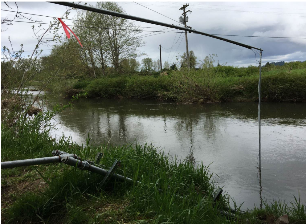
Figure 4. A boom-arm probe deployment on the Newaukum River near Chehalis, adjacent to a slant pipe deployment.
