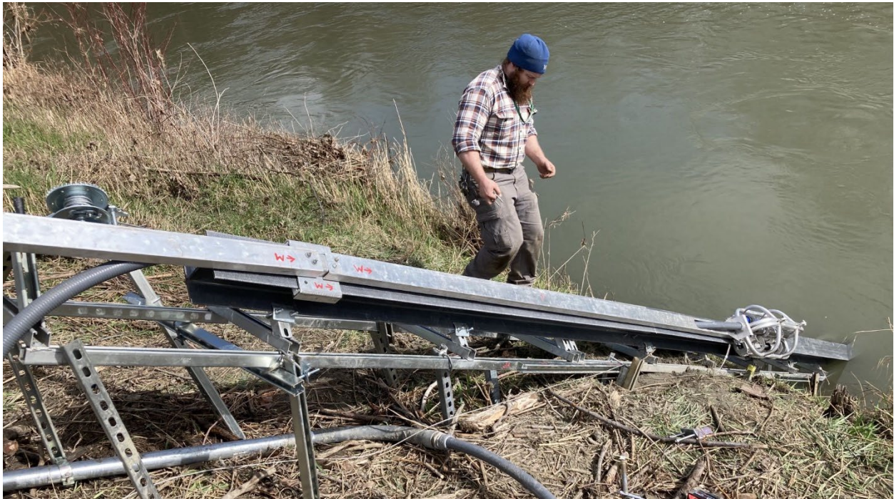
Figure 3. Probe shuttle and an I-beam with an improved anchor frame at the Stillaguamish River at Blue Stilly Park, March 23, 2023.
