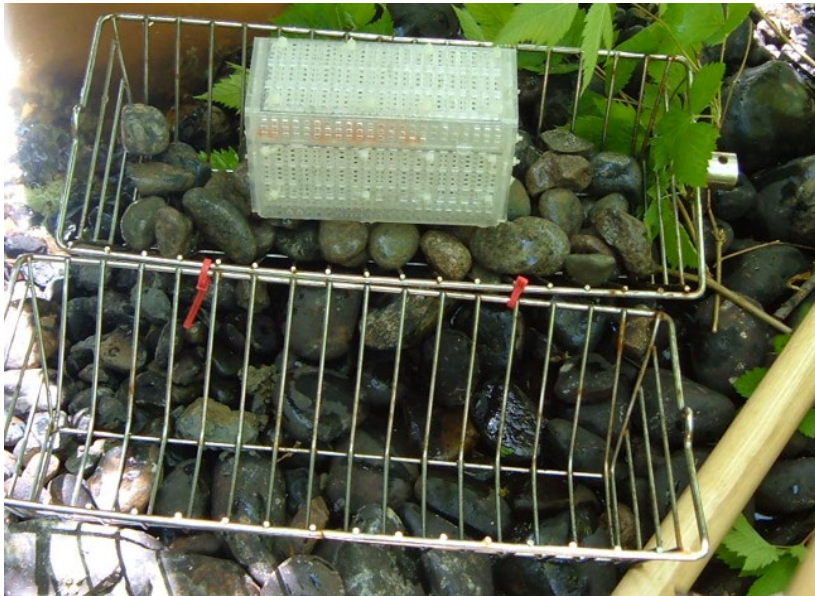
Figure 23. Fish hatchbox used to measure the health of a stream for target fish species.
