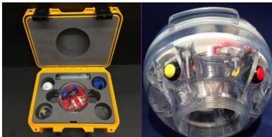
Figure 19. An example of an active sampling device that collects water in situ. Device in a waterproof case (left) and a closeup of the device (right).
