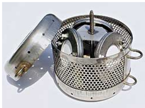
Figure 20. POCIS passive sampling device (USGS and EST).
