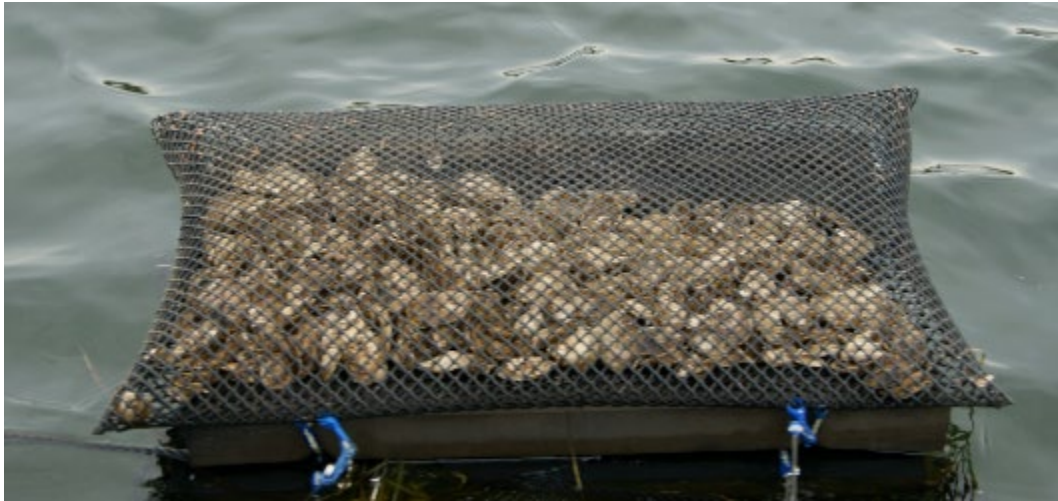
Figure 24. Example of a mesh bag for housing shellfish bioassays.
